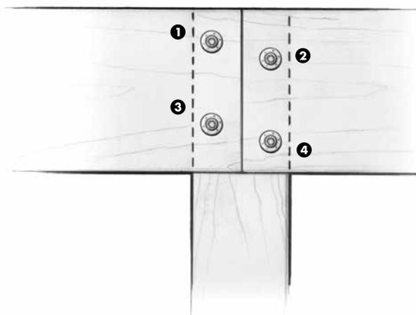
1. Install first screw 1" in from the edge of the post and 2" (+/- 1/4") from the top of the beam
